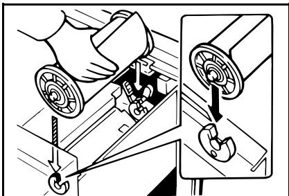
**5** Insert the paper edge of the master roll under the arrow mark (1) until you can see the leading edge under the transparent cover.
