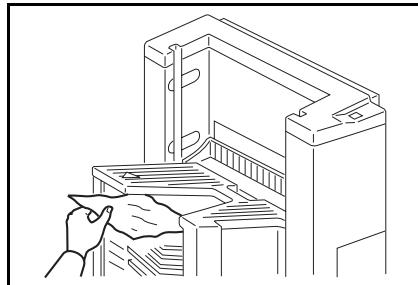
**2** Open the non-sort tray. If you cannot remove misfed paper, remove paper under the non-sort tray.
