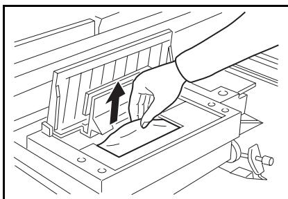
**4** If you could not remove the misfed master in steps 2 and 3, take out the drum and remove the misfed master from the inside.
