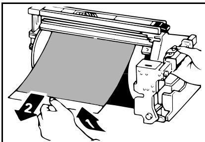
**3** Remove paper that is stuck to the drum.
