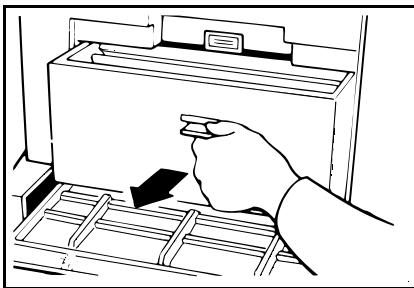
**3** Reinstall the master eject box. Push in the box until it touches the inside bracket.
