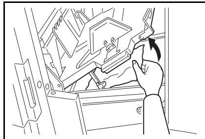
**3** While lifting the non-sort tray, lower the knob to the right. Then, close the non-sort tray.
