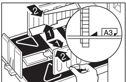
**8** If you want to use A4, 8 1/2" x 11" or smaller paper, lift the small size paper delivery end plate and move it to match the print paper size.
