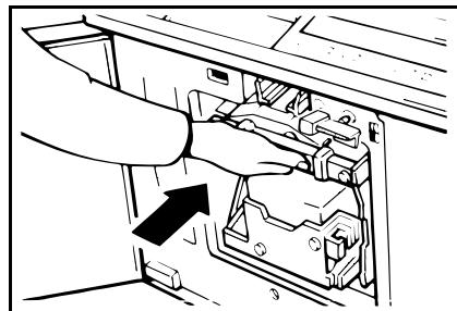
**9** Lower the drum unit lock lever.
