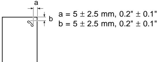
**Stapler Capacity:**50 sheets (64 g/m<sup>2</sup>, 17.1 lb)40 sheets (80 g/m<sup>2</sup>, 20 lb)42 sheets (75 g/m<sup>2</sup>, 20 lb)**Staple replenishment:** Cartridge exchange (5,000 pieces/cartridge)**Dimensions (only sorter stapler):**
