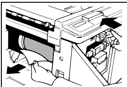
**4** If you cannot remove the mis-fed paper, pull out the drum unit after confirming that the lamp is green, and remove the misfed paper from the drum.
