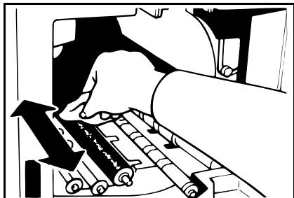
**4** Remove with a clean cloth any ink that has accumulated on the trailing edge of the drum unit.
