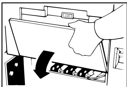
**2** Take out the master eject box and remove the used masters.
