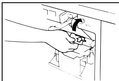
**4** Pull out the drum unit handle while pressing the release bar inside the green handle.
