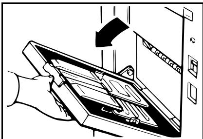
**6** Lift the paper delivery end plate and move it to match the print paper size.
