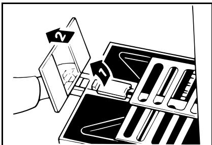
**7** Lift the paper delivery side plates and adjust them to the paper size.
