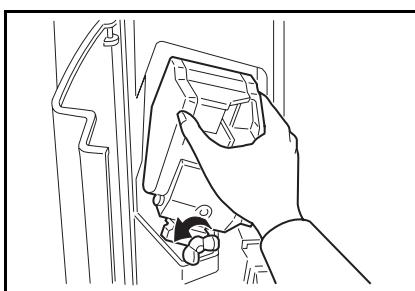
**3** While pushing the stopper down, push the knob to your side. Then, open the stapler unit cover.
