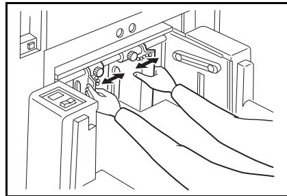
**7** Secure the side plates with the screws.
