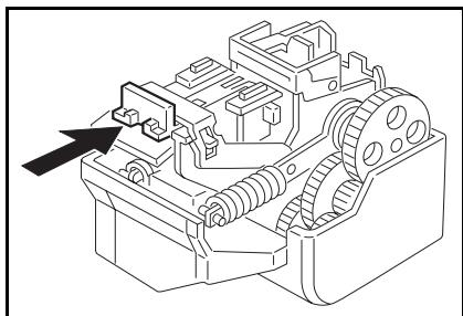
**6** Return the stapler unit to its original position and secure the screw.
