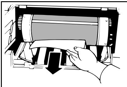
**3** If the paper is completely wrapped around the drum, peel off the edge of the paper. Then, close the master eject unit and press the drum rotation button until the lamp turns green again. And then, open the master eject unit and remove the misfed paper.
