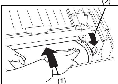
**7** Press the master cut button to cut the leading edge of the master roll.
