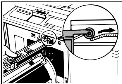
**8** Slide in the drum unit until the drum unit locks in position.
